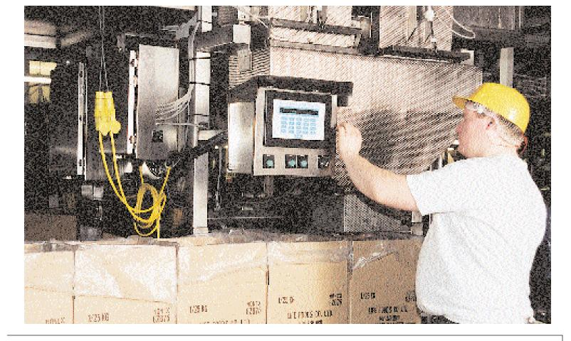
An operator controls the volume and speed of the machine that takes the characteristics of the frozen vegetables into account. The new high volume machine can be programmed ahead of the run and controlled from the panel.
